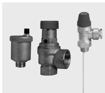
Valves Kit (421600) consisting of: automatic air relief valve, 1.5 bar safety valve, 90 ° C thermal relief valve
